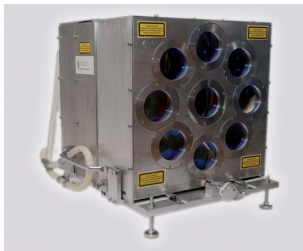
Fig. 10 Fielded brass board 9-VCSEL model.
