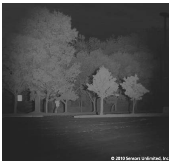
Fig. 6. Night-time image under 2~3W VCSEL-based illumination at 976nm. An InGaAs-based camera was used to capture the image.
